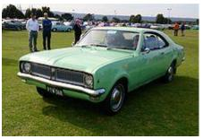
Most mechanical specifications were carried over from the HT series with the exception of the non 350 Monaro GTS which featured a softened suspension tune to make a for a smoother ride. The manual HG GTS retained the stiffer suspension of the HT GTS 350. Thicker front disk brake rotors featured across the range.
