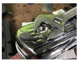
Screw in the cap and reinstall rocker cover back on the motor. I put some water in the rocker cover to check for leaks....found none.
